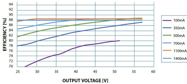
**EFFICIENCY vs OUTPUT VOLTAGE (277VAC)**
