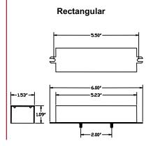
Dimensions for unit with stud mounting
