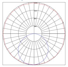
$\label{eq:maximum Candela = 1374 Located At Horizontal Angle = 270, Vertical Angle = 5 \ \#\ 1 - Vertical\ Plane\ Through\ Horizontal\ Angles\ (270 - 90)\ (Through\ Max.\ Cd.)$ # 2 - Horizontal Cone Through Vertical Angle (5) (Through Max. Cd.)
