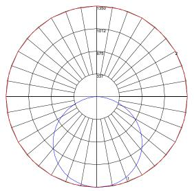
$\label{eq:maximum Condela} \begin{tabular}{ll} Maximum Candela = 1349.9 & Located At Horizontal Angle = 0, Vertical Angle = #1 - Vertical Plane Through Horizontal Angles (0 - 180) (Through Max. Cd.) #2 - Horizontal Cone Through Vertical Angle (0 ) (Through Max. Cd.) \\ \end{tabular}$
