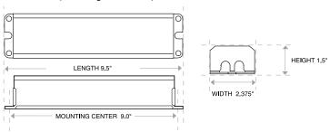
I-42-LOL has same basic specs, but different wiring connections than shown. These are custom built for Lightolier fixtures. No dedicated LOL specs available from lota.
