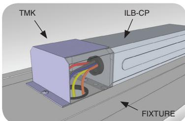
When top-mounting "B" configuration ILB-CP units, the TMK-80 is used to cover the exposed wiring that goes from the battery pack into the fixture.
