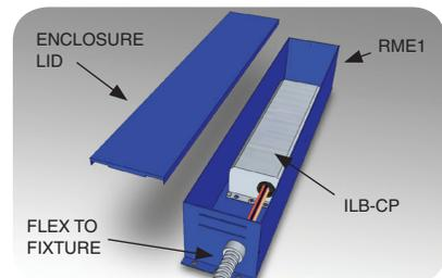
The RME1 enclosure accepts "B" configuration ILB-CP units for remote mounting. The ILB-CP is secured within the enclosure and wiring is routed through the 2 ft. of flexible conduit for connecting to the fixture. Can be used in conjunction with the TBMK for grid ceiling mounting.
