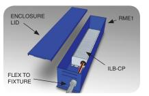
The RME1 enclosures accepts "B" configuration ILB-CP units for remote mounting. The ILB-CP is secured within the enclosure and wiring is routed through the 2 ft. of flexible conduit for connecting to the fixture. Can be used in conjunction with the TBMK for grid ceiling mounting.
