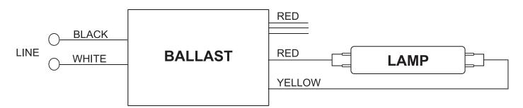
Ground case in accordance with the National Electric Code. Cap and insulate any unused red wire individually.
