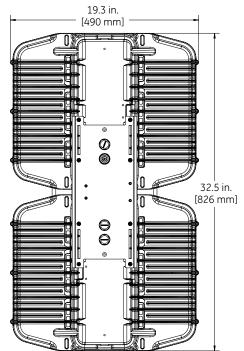
Max Weight with Rotatable Bracket Max Weight Configuration Single Fixture 120-277V 21 lbs. max 25 lbs. max Single Fixture 347/480V 23 lbs. max 27 lbs. max Double Fixture 120-277V 45 lbs. max N/A Double Fixture 347/480V 49 lbs. max N/A 1 3.5 in. [89 mm]
