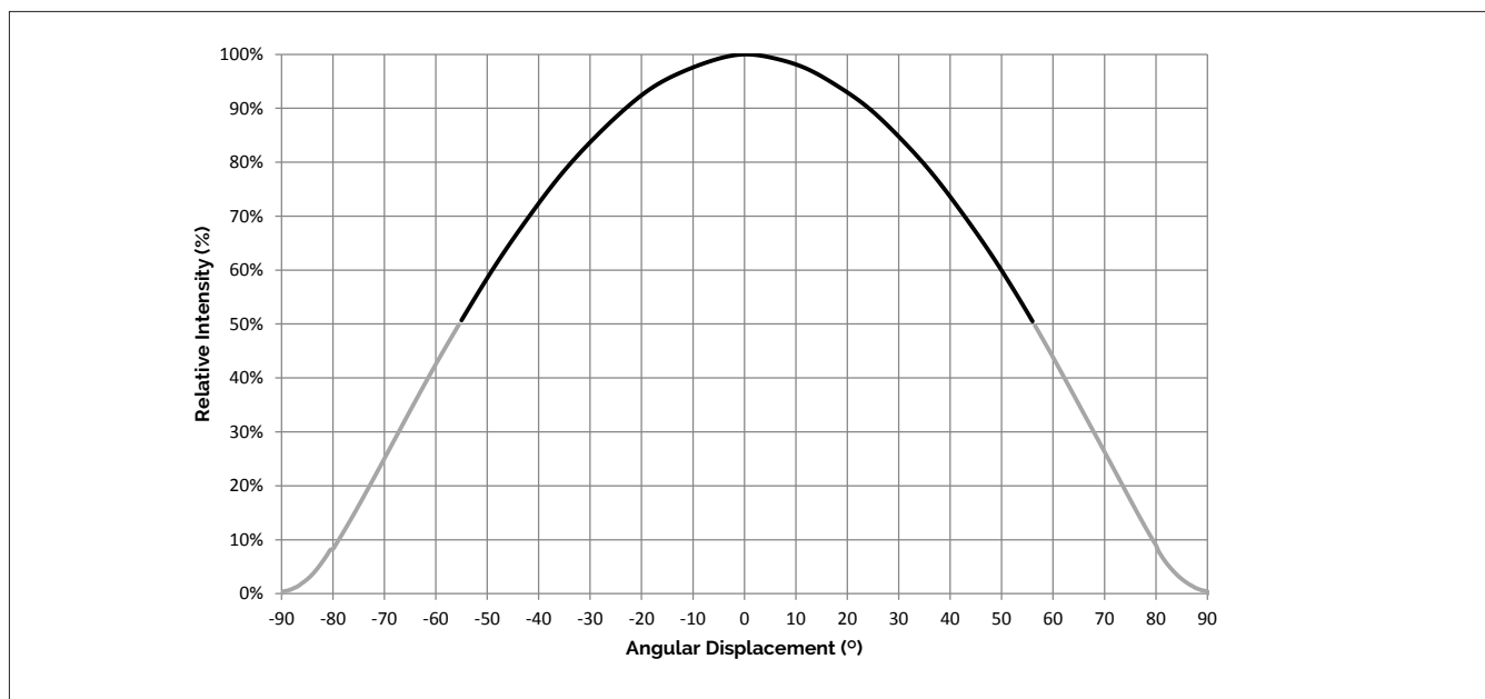
Figure 15: Typical Spatial Radiation Pattern
