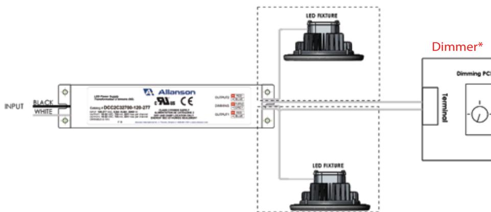
\* Order Dimmer Part #26-003 with the Dimming Power Supply (DCC2C32700-120-277).
