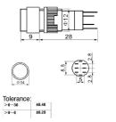
Recommended hole size for installation: Ø12mm
