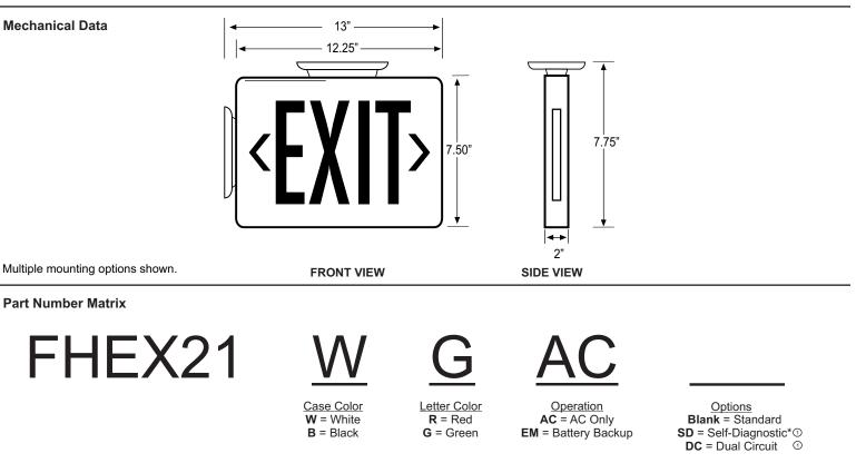
\*Self-Diagnostic option tests the fixture every 30 days for 15 minutes and once every 12 months for a full 90 min discharge test. After each test the battery is recharged automatically and the unit returns to normal operating mode. Any problems found during or after the test are reported through the user interface.
