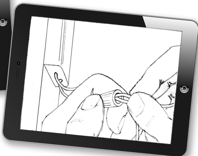
Step 2 Install Tetra 24-volt power supply
