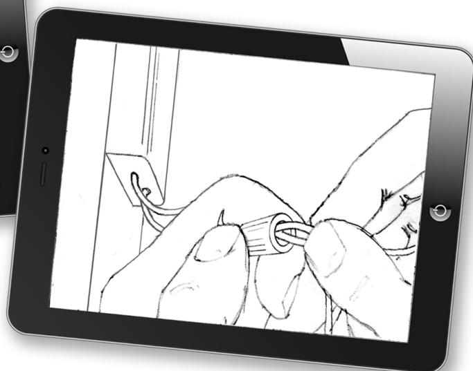
Step 2 Install Tetra 24-volt power supply
