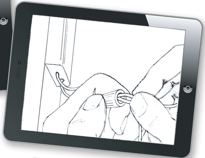
Step 2 Install Tetra 24-volt power supply
