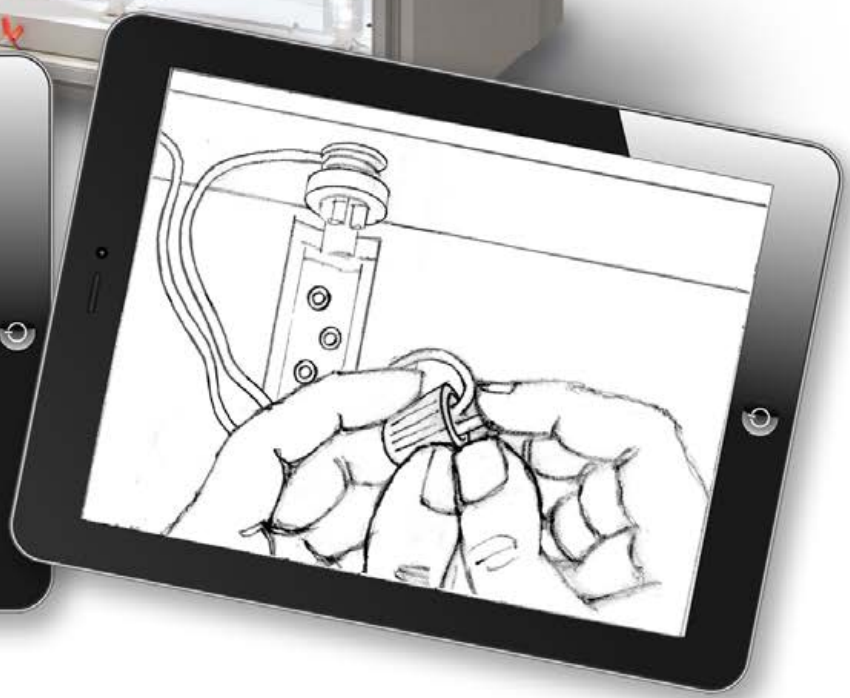
Step 4 Connect wires to LED bars and back to power supply
