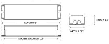
I-42-EMKV has same basic specs, but different wiring connections than shown. These are custom built for Kurt Versen fixtures. No dedicated EMKV specs available from lota.
