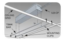
Use the TBMK mounting kit to remote mount flexed units within a grid ceiling. The ILB-CP is secured to the bars of the TBMK via mounting clips. The bars then mount to the T-bars of the ceiling grid. The flexible conduit of the ILB-CP connects to the fixture. O RME1 Remote Mounting Enclosure
