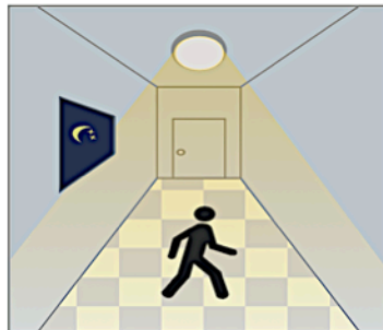
With insufficient daylight, when motion detected, light ON.
