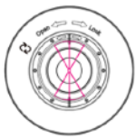
Aisle/Corridor application: Split the lens cover into aisle type.
