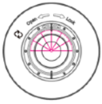
Semi-sphere application: Split the lens cover into Semi-circle type.
