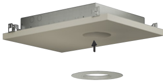
1. Fasten mud frame to ceiling.
