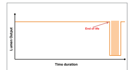
D. End of Life Power Supply Indicator
