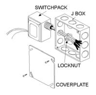
All connections are made via pigtails with twist-on wire connectors.
